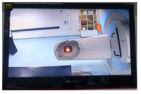
Fig. 2.4: shows the Synergy's gantry position during the radiation survey procedure (taken from the camera), which is the position at which the primary radiation is face to face to the control console.
